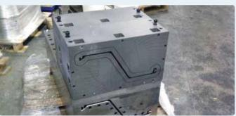
3 Next, the fiber architecture enters MPG's proprietary injector for fiber wet out. MPG's injector (top) is modular in design and is completely independent of the die (bottom). The injector is made to mate with the parting lines of the die. Both require tight tolerances (within ±0.001 inch/ ±0.025 mm) because PU lacks the resilience necessary to conform to obstructions.
