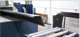
8 The Gulf profiles are pultruded at a rate under 2-ft/min (0.61m/min) An automatic, flying cut-off saw cuts the profiles to the specified length for each job. 🔳
