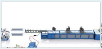
6 An artist's conception of Martin Pultrusion's dedicated Gulf machine (with the meter/mix components cut off, bottom). A 6 ft/1.8m space has been added between the die and the first clamp puller (with air knives) to provide an extra 1 to 2 minutes of ambient cooling time. If enough heat isn't drawn out of the profile, the clamp pullers have a hard time gripping the part.
