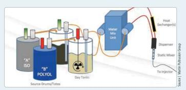
4 A two-part meter/mix unit provides a steady stream of PU to the injector. It's critical that resin is delivered without any pulsation or variation in flow or pressure to the injector. A series of complex internal geometries enable the injector to create the necessary pressure for fiber wet out.
