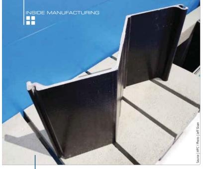
I The PURIoc sheet pile system uses a series of corrugated, interlocking piles to form a watertight wall. Each sheet pile profile is Z-shaped with a depth section of 8.5 inches/216 mm, a wall thickness of 0.25 in/6.35 mm and a width of 18 inches/457 mm (length depends on application).
