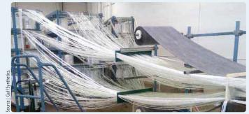
Approximately 900 ends of the heaviest weight roving (56 yield) flow into Gulf's sheet pile. Also incorporated are two layers of biaxial stitched fabric, one on the bottom and one on the top. The resulting pultrusion has a glass loading of approximately 78 percent by weight. High glass loading is typical for PU pultrusions and can range from 75 to 80 percent by weight.
