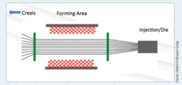
2 Prior to forming, the fiber is run through 3 to 4 seconds of infrared heat (approximately 120°F/49°C). Because PU reacts to moisture, fiber drying is critical. Excess moisture can cause blistering on the pile profile surface. The fiber architecture is fully formed before it enters the injector.
