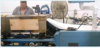
5 MPG included two removable inserts in the Gulf die to allow for different wall thicknesses. When competing against a lower cost resin like PVC, the inserts can be switched out to produce a thinner profile. At the exit end of the die, a cooling zone is required to act as a heat sink. It's not uncommon for MPG to see heat zones between 425°F/218°C and 450°F/232°C through the die. The cooling zone can drop the temperature by as much as 125°F/52°C.
